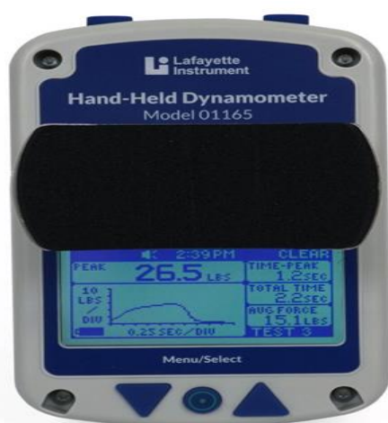
Figure 5: Lafayette Handheld dynamometer (Adopted from Celik et al., 2012).
